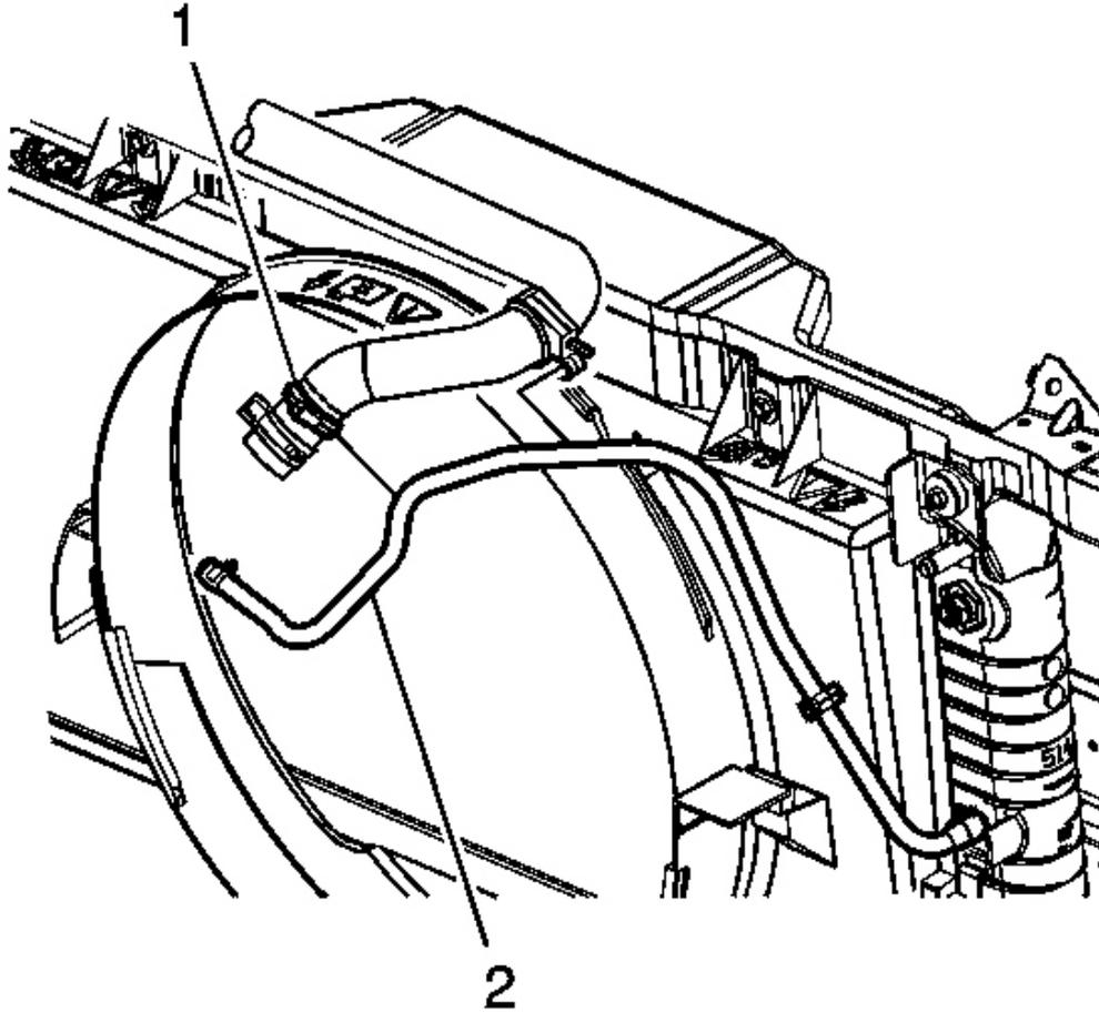
**Fig. 32: Radiator Vent Inlet Hose**
