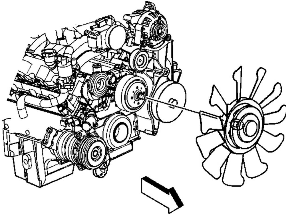
**Fig. 50: View Of Fan Assembly**
