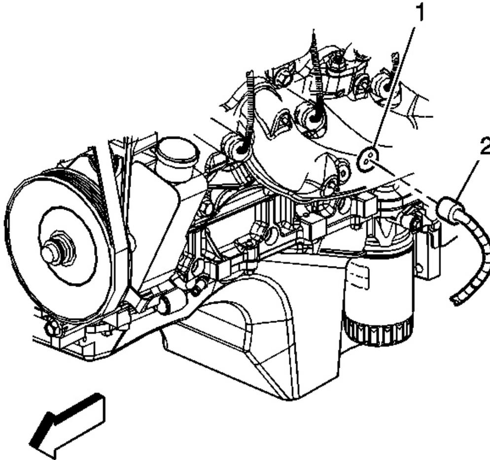
**Fig. 109: Engine Coolant Heater Cord Electrical Connector & Coolant Heater**
