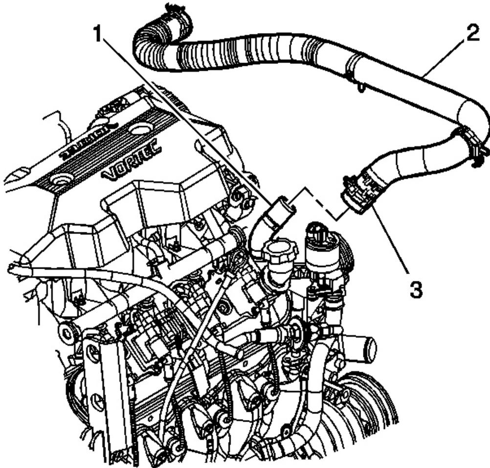
**Fig. 26: Radiator Hose & Engine (Inlet)**
