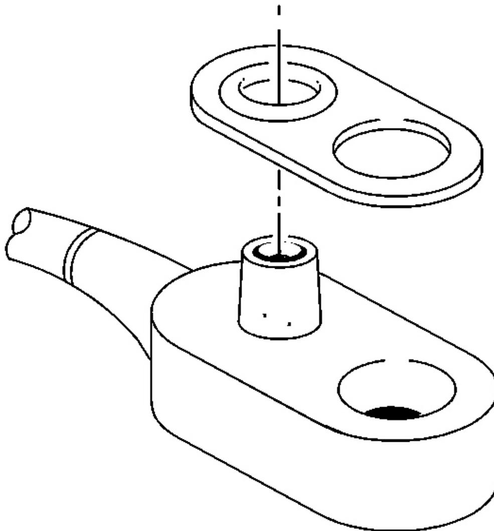
**Fig. 66: Pipe & Cover Gasket**
