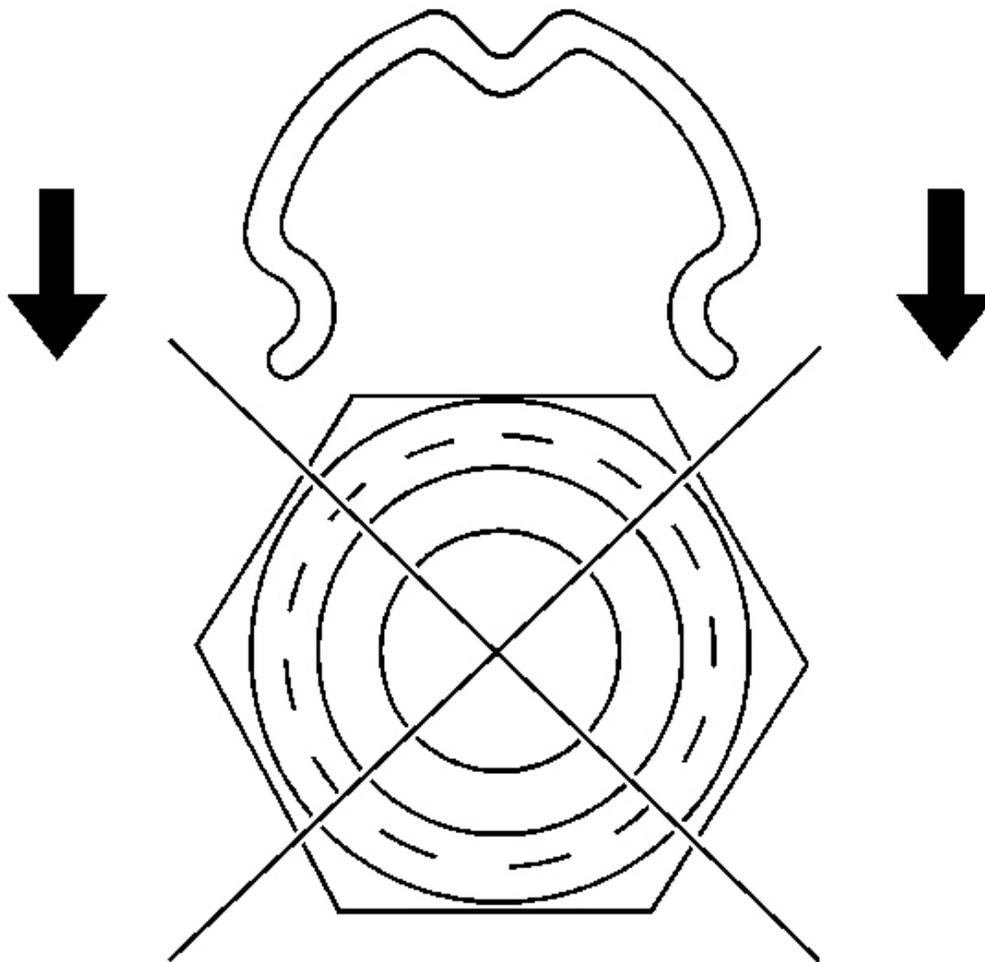
**Fig. 35: Do Not Install Retaining Ring In This Manner**
