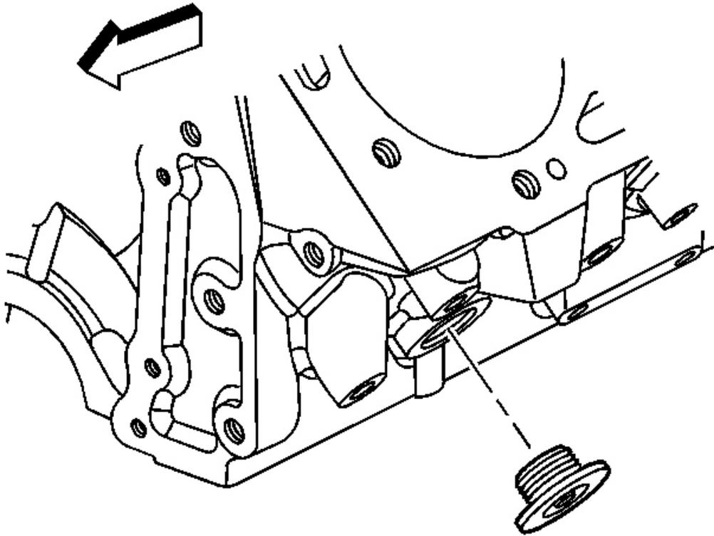
**Fig. 6: Left & Right Engine Block Coolant Drain Hole Plugs**
