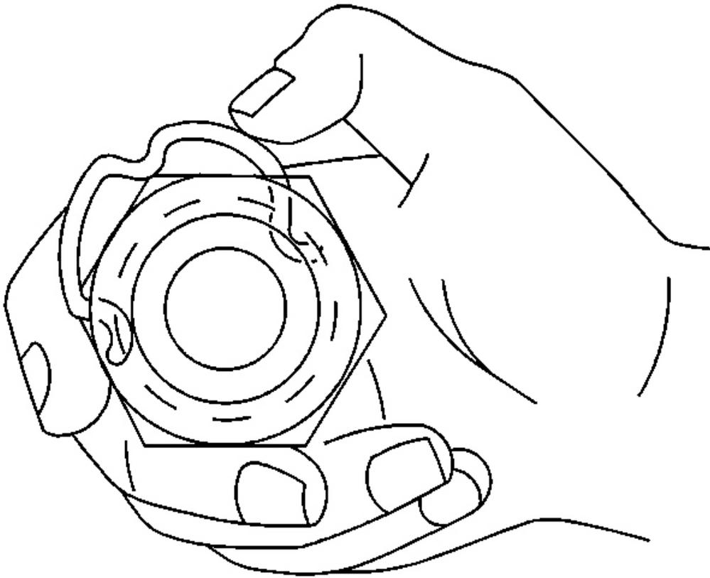
**Fig. 37: Rotating Retaining Ring Around Connector**
