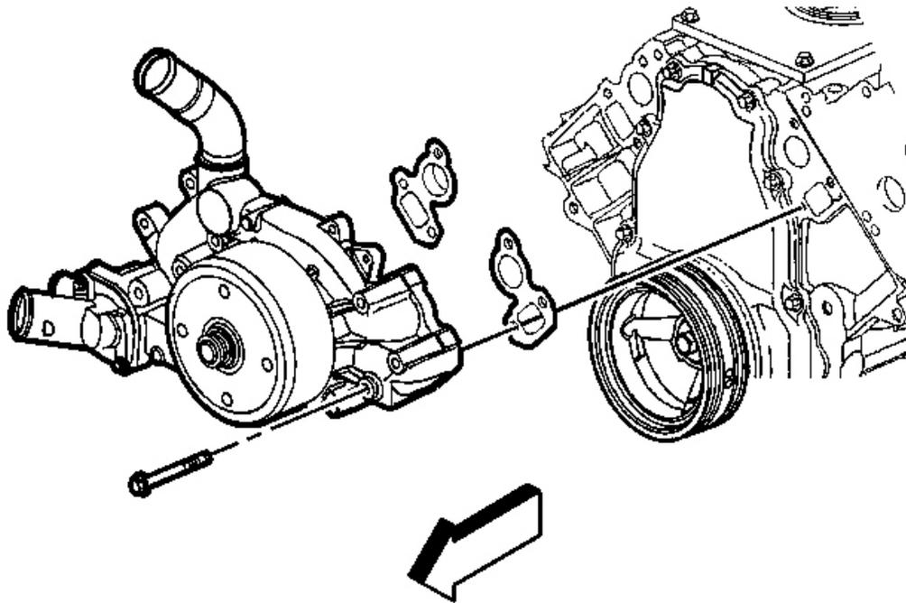
**Fig. 79: Water Pump & Bolt**
