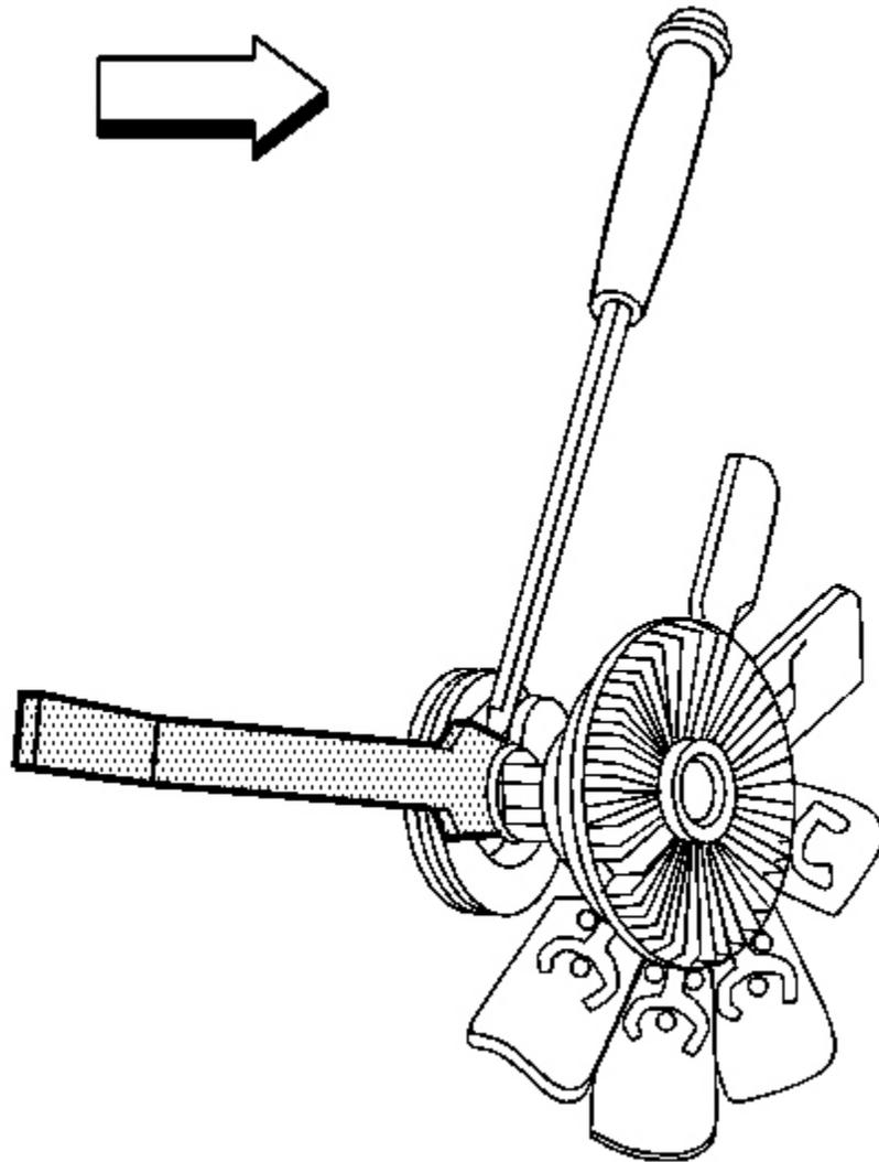
**Fig. 51: Installing J 46406 To Fan Clutch**
