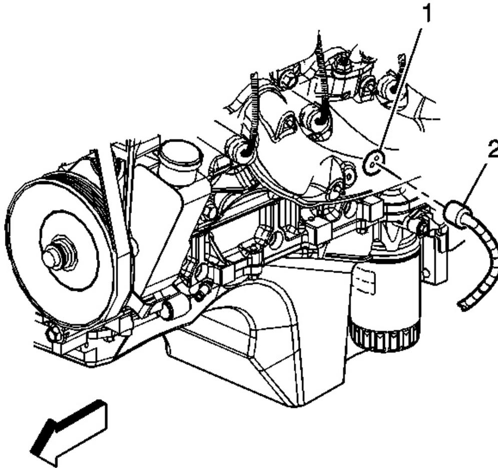
**Fig. 106: Engine Coolant Heater Cord Electrical Connector & Coolant Heater**
