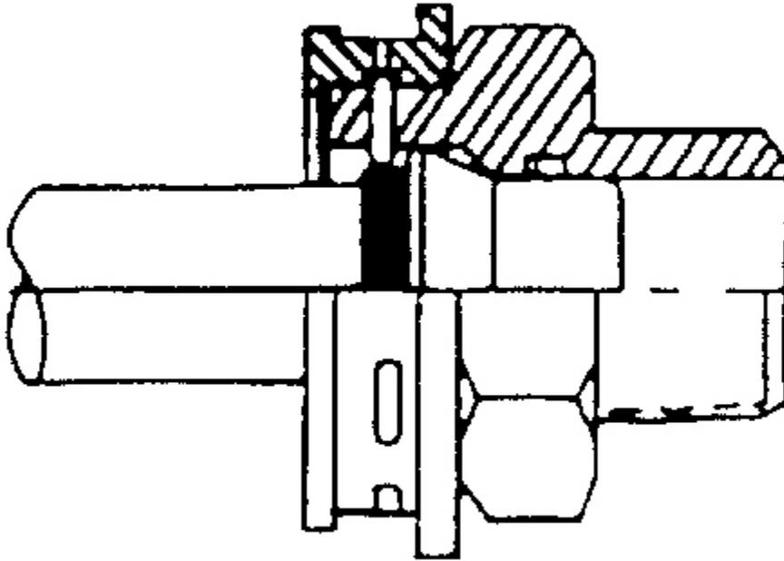
**Fig. 40: Inserting Plastic Cap Onto Fitting**
