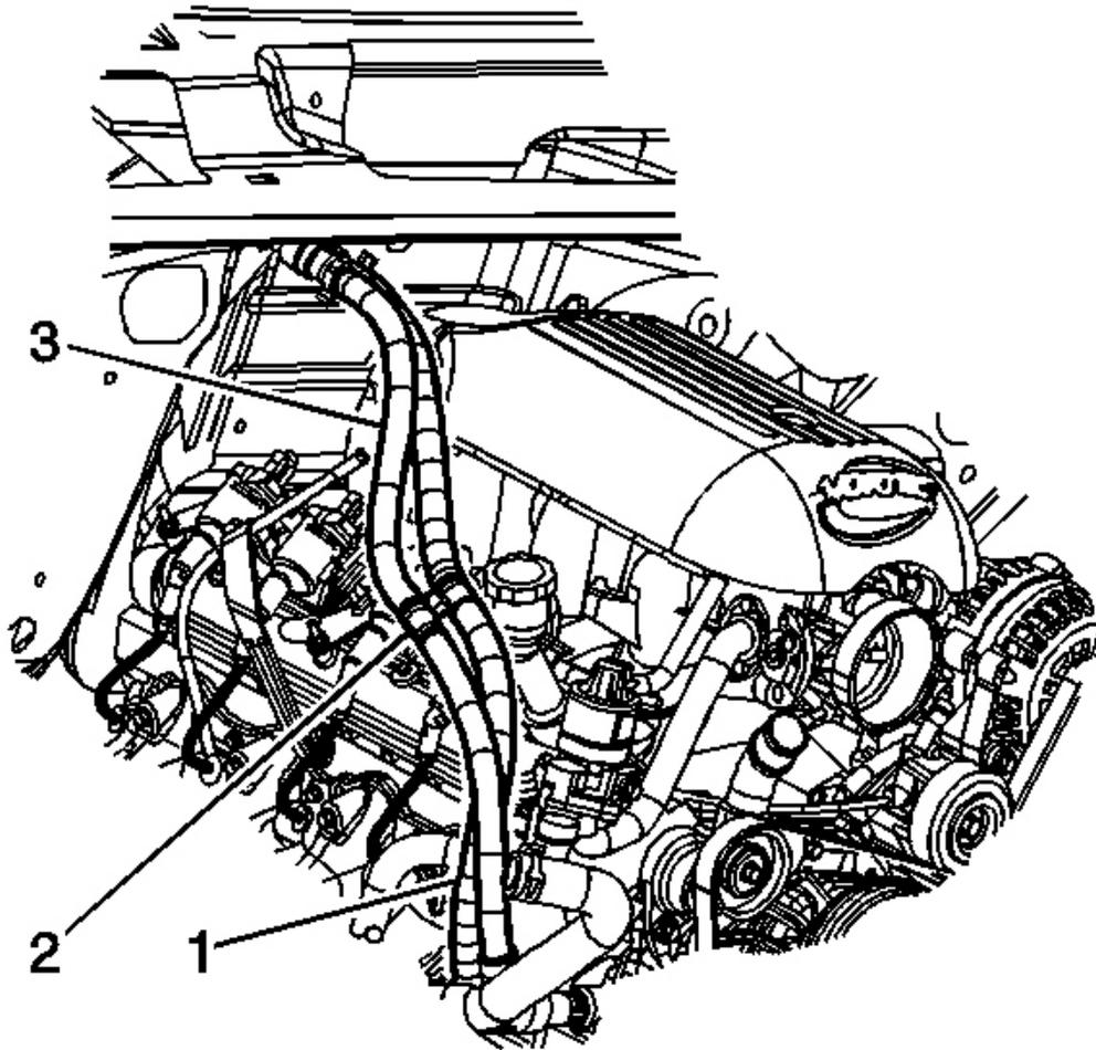
**Fig. 21: Heater Hose & Mounting Clip**
