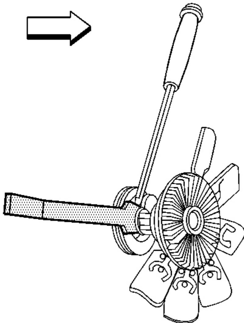
**Fig. 46: Installing J 46406 To Fan Clutch**
