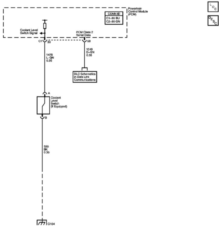
**Fig. 1: Engine Cooling Schematics**
