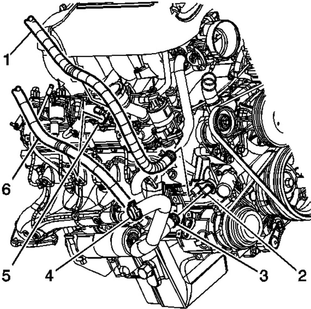
**Fig. 20: Surge Tank Hose & Engine (Outlet)**
