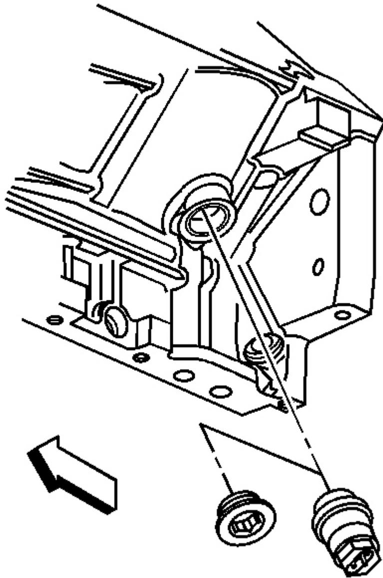
**Fig. 105: Installing Engine Coolant Heater In Place Of Drain Plug**
