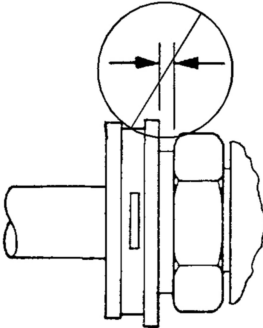
**Fig. 41: Ensuring That No Gap Is Present Between Cap & Fitting**
