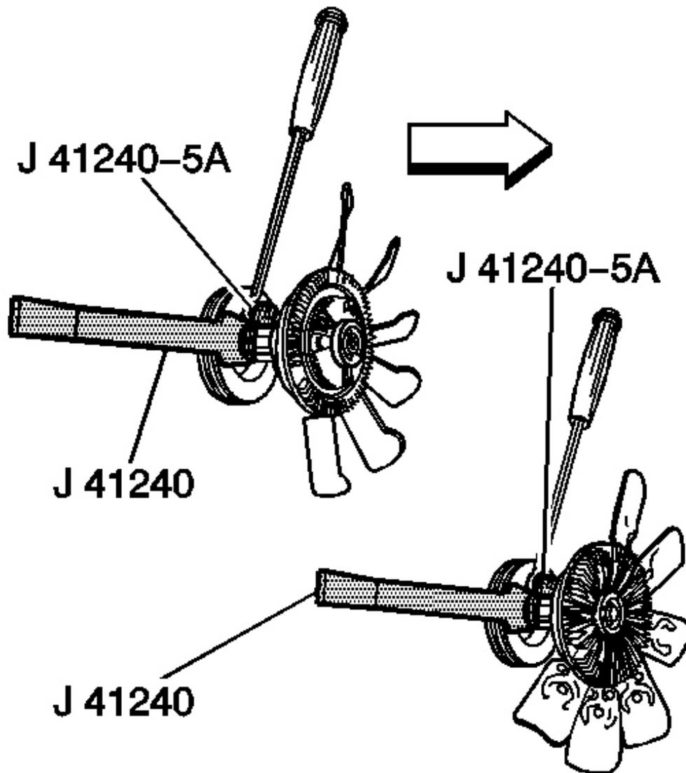
**Fig. 52: Using Special Tools For Fan Clutch**
