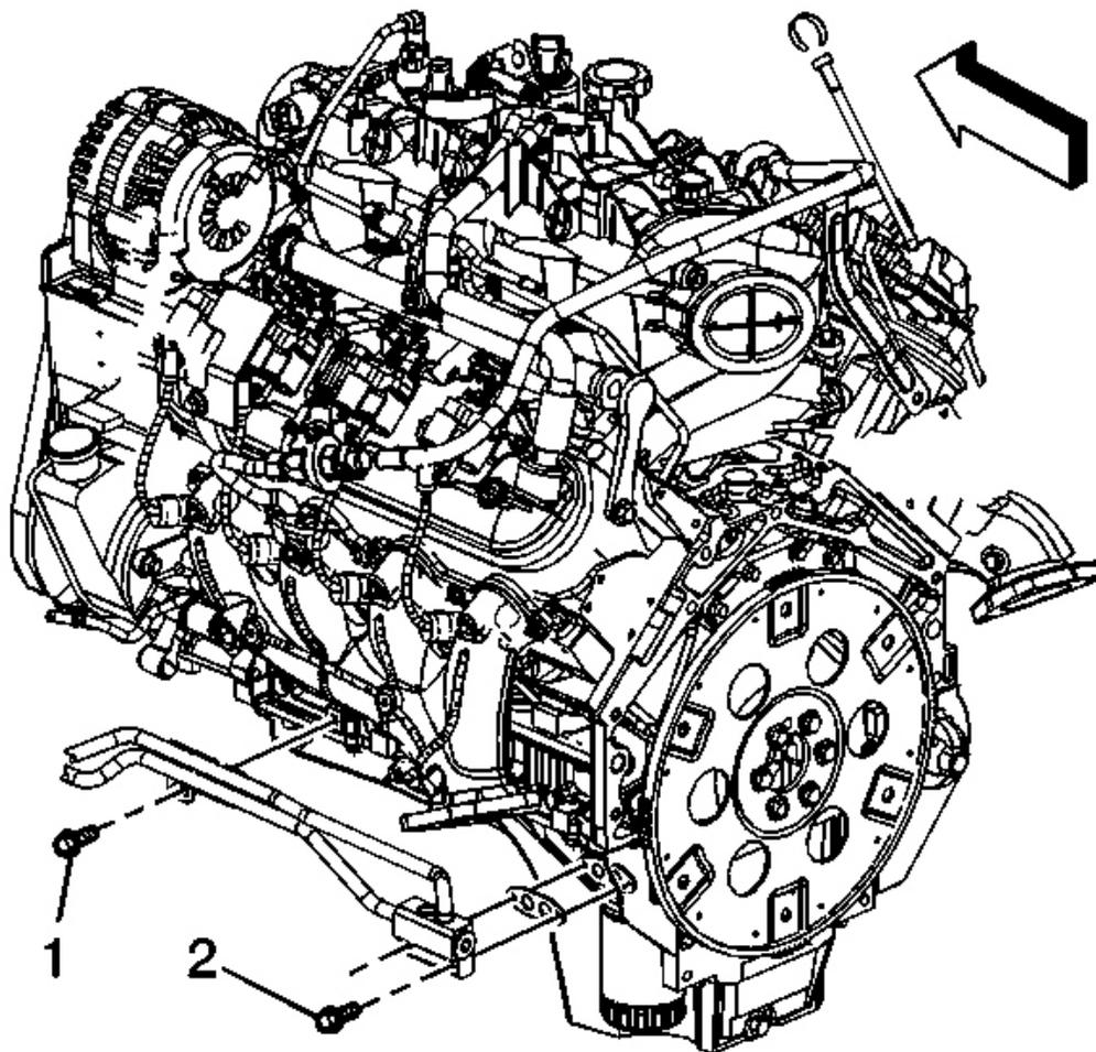
**Fig. 44: Oil Cooler Hose Bracket Bolt & Adapter Bolts**
