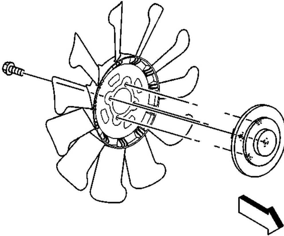
**Fig. 55: Fan Clutch & Fan Blade**
