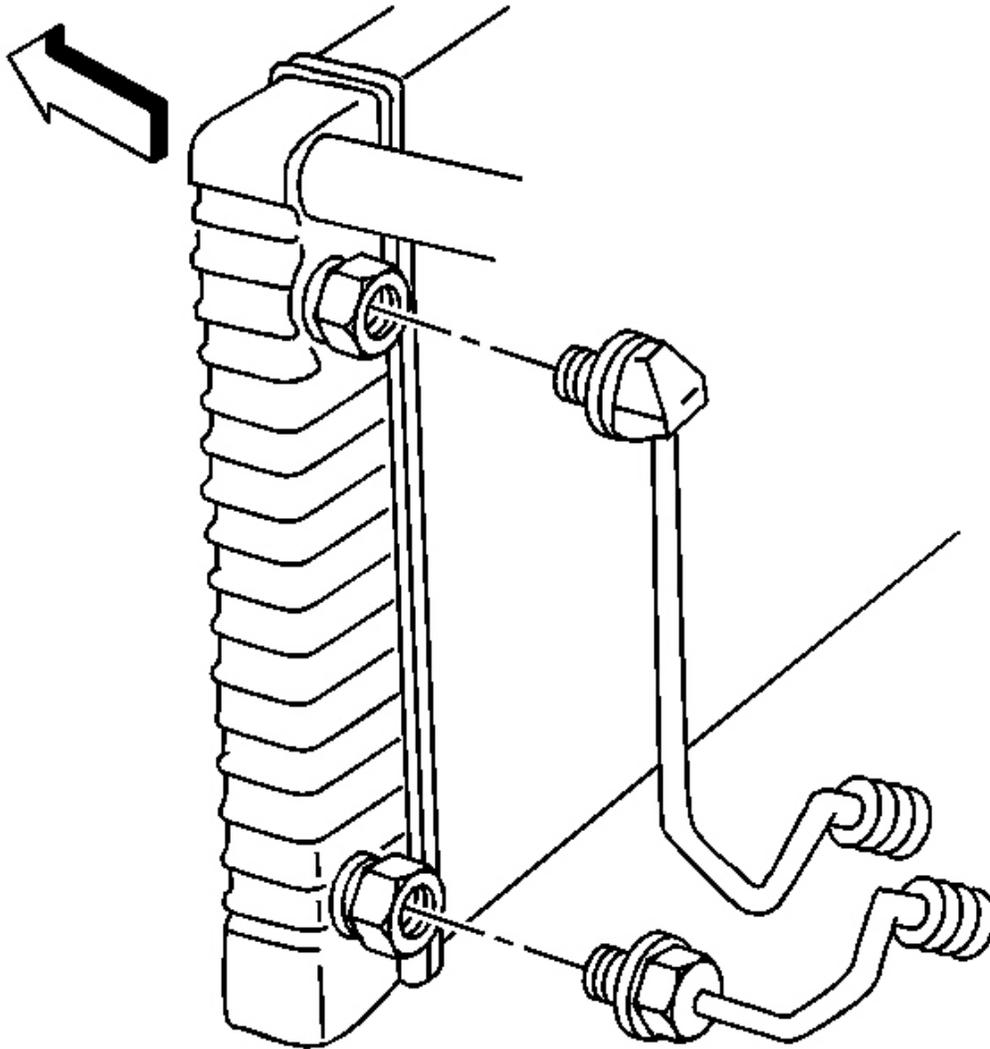
**Fig. 39: Engine Oil Cooler Line**
