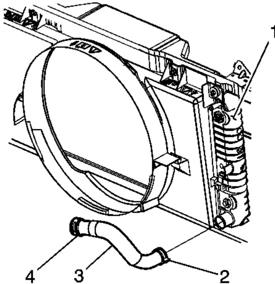
**Fig. 93: Radiator Hose & Radiator (Outlet)**
