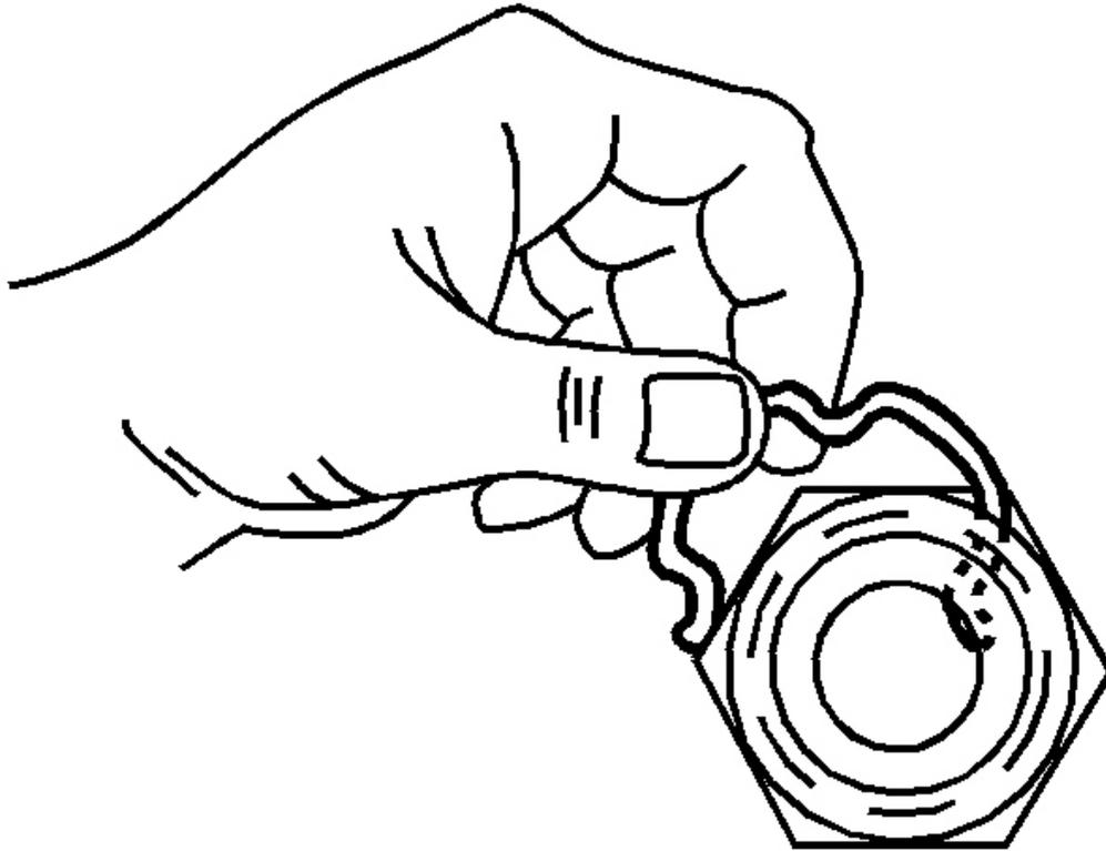
**Fig. 36: Hooking Retaining Ring**
