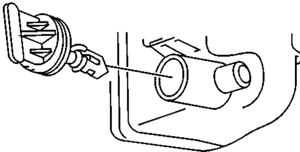
**Fig. 86: Radiator Drain Cock**
