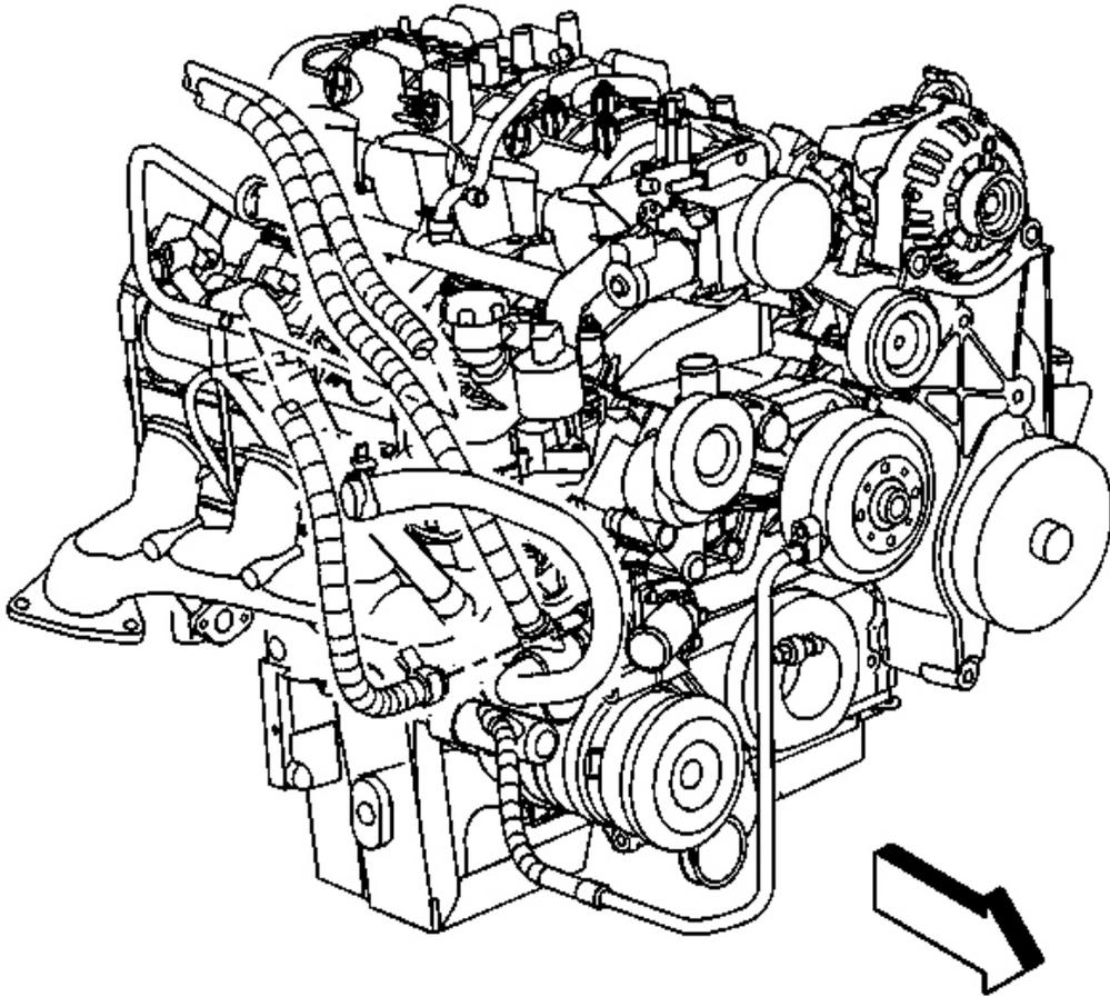
**Fig. 77: Heater Inlet Hose**
