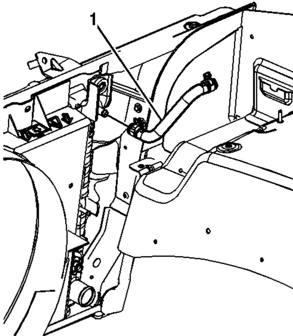
**Fig. 99: Surge Tank Hose & Radiator (Inlet)**
