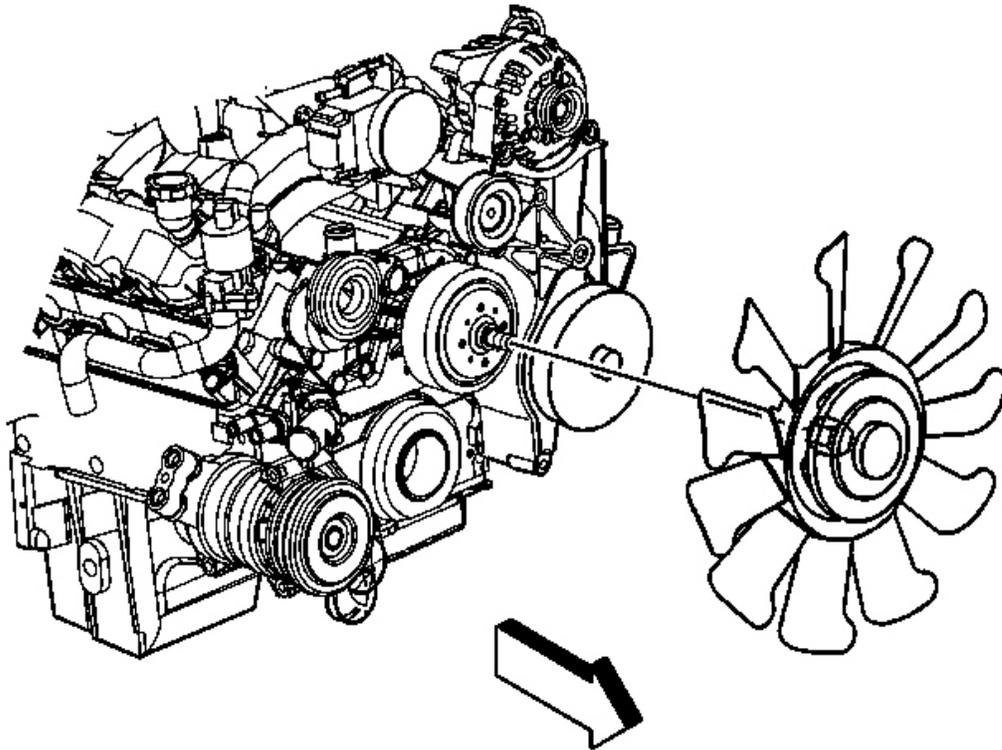
**Fig. 53: View Of Fan Assembly**
