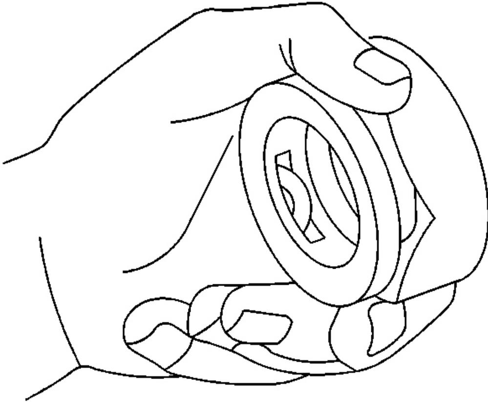
**Fig. 38: Ensuring Retaining Ring Ears Are Seen From Inside Of Connector & Retaining Ring**
