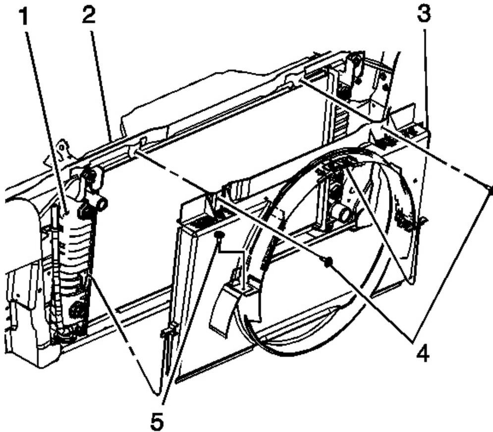
**Fig. 89: Identifying Fan Shroud**
