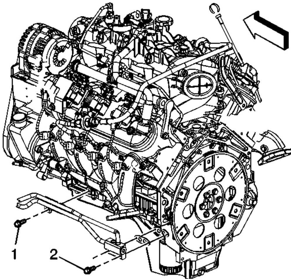
**Fig. 104: Oil Cooler Hose Bracket Bolt & Adapter Bolts**
