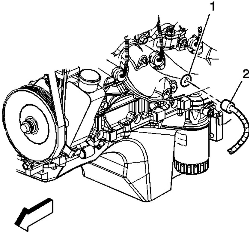
**Fig. 112: Engine Coolant Heater Cord Electrical Connector & Coolant Heater**
