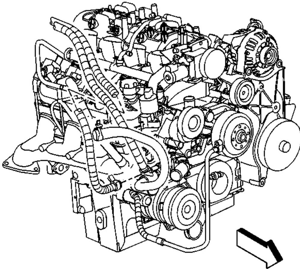
**Fig. 80: Heater Inlet Hose**
