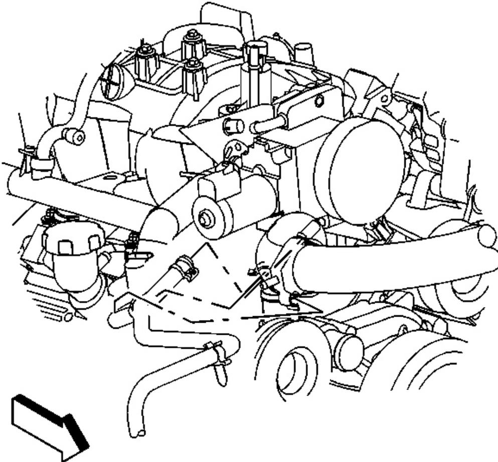
**Fig. 73: Vent Inlet Hose At Throttle Body**
