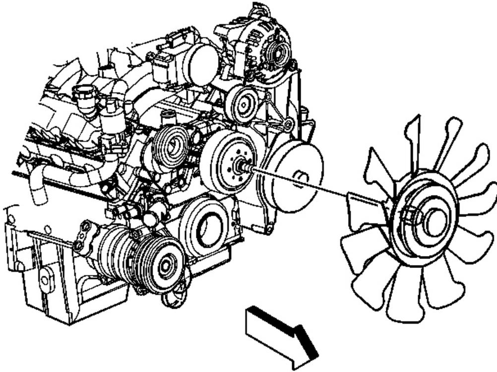
**Fig. 56: View Of Fan Assembly**
