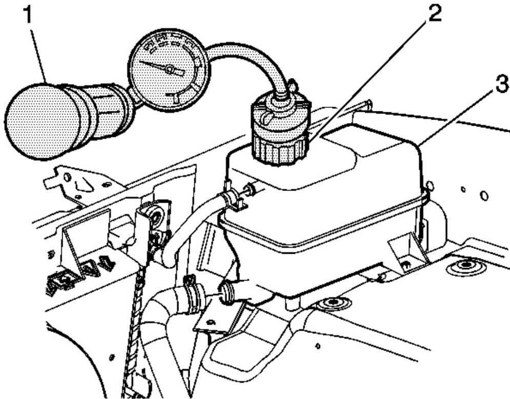
**Fig. 5: Using J 24460-01 With J42401 To Apply Pressure To Cooling System**
