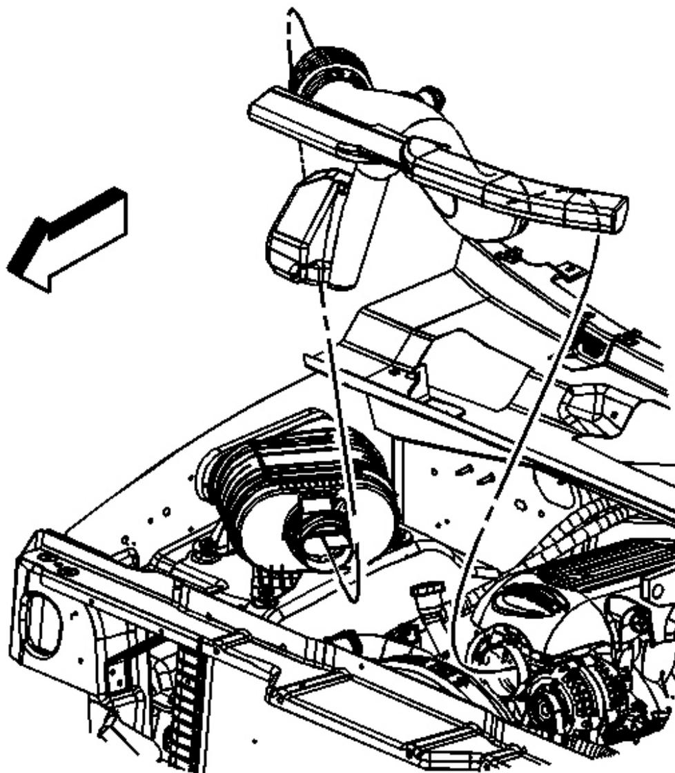
**Fig. 61: Air Cleaner Outlet Duct**
