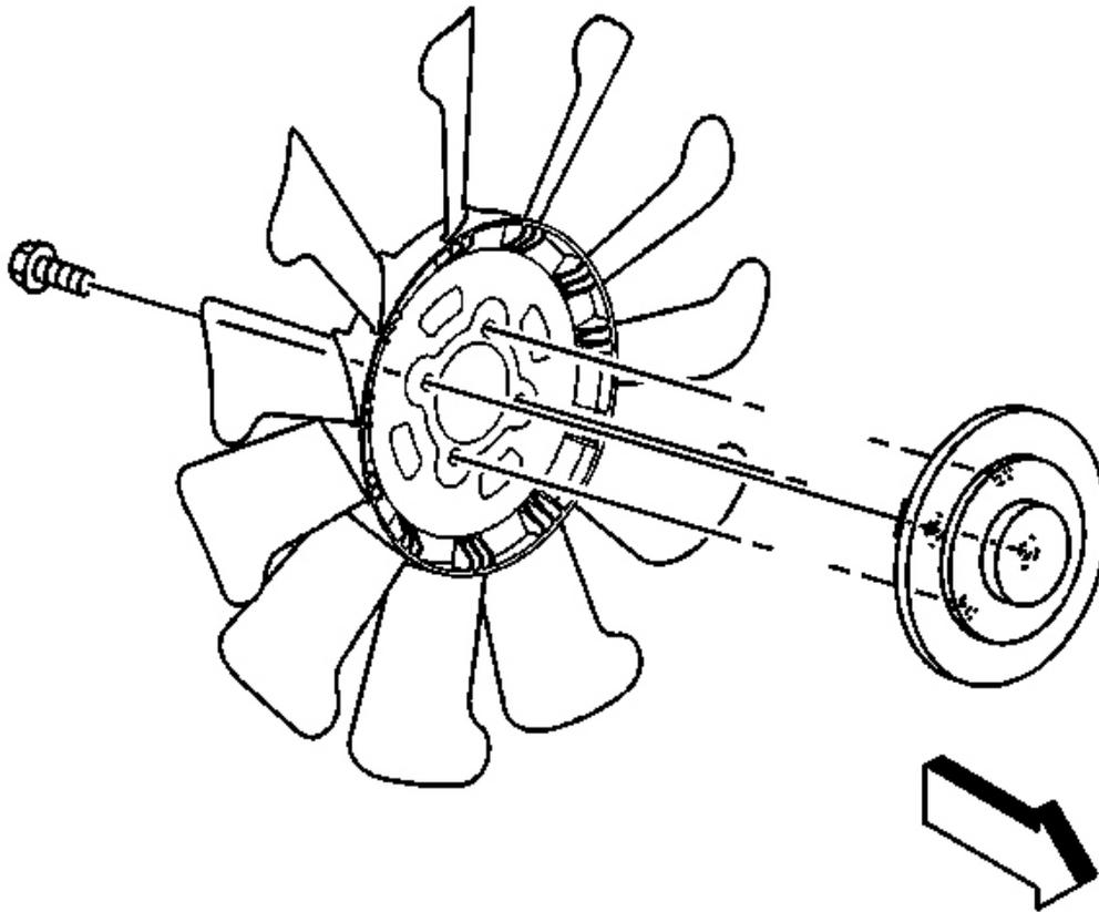
**Fig. 54: Fan Clutch & Fan Blade**
