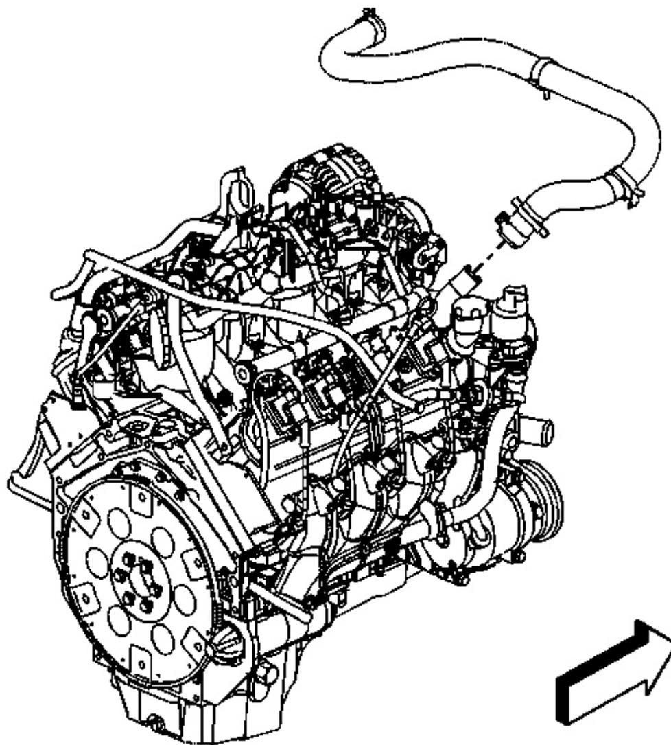
**Fig. 74: Inlet Hose & Water Pump (4.8, 5.3, & 6.0L)**
