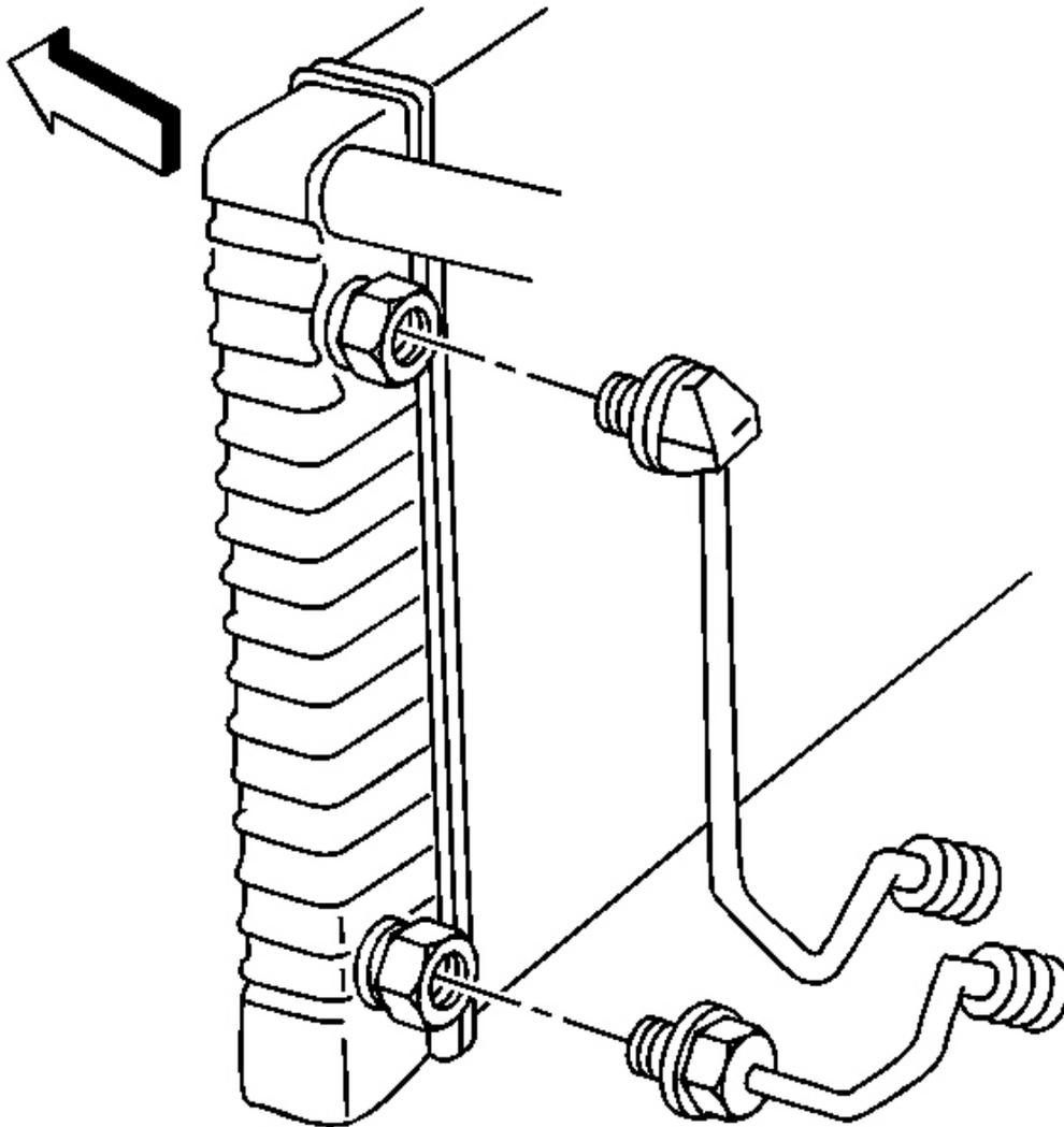
**Fig. 34: Engine Oil Cooler Line**
