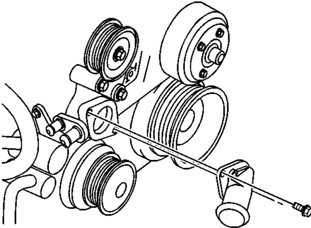
**Fig. 59: Water Pump Inlet & Thermostat Housing**
