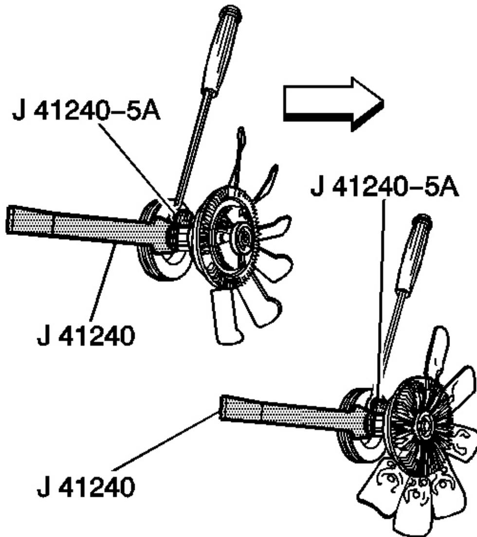
**Fig. 57: Using Special Tools For Fan Clutch**
