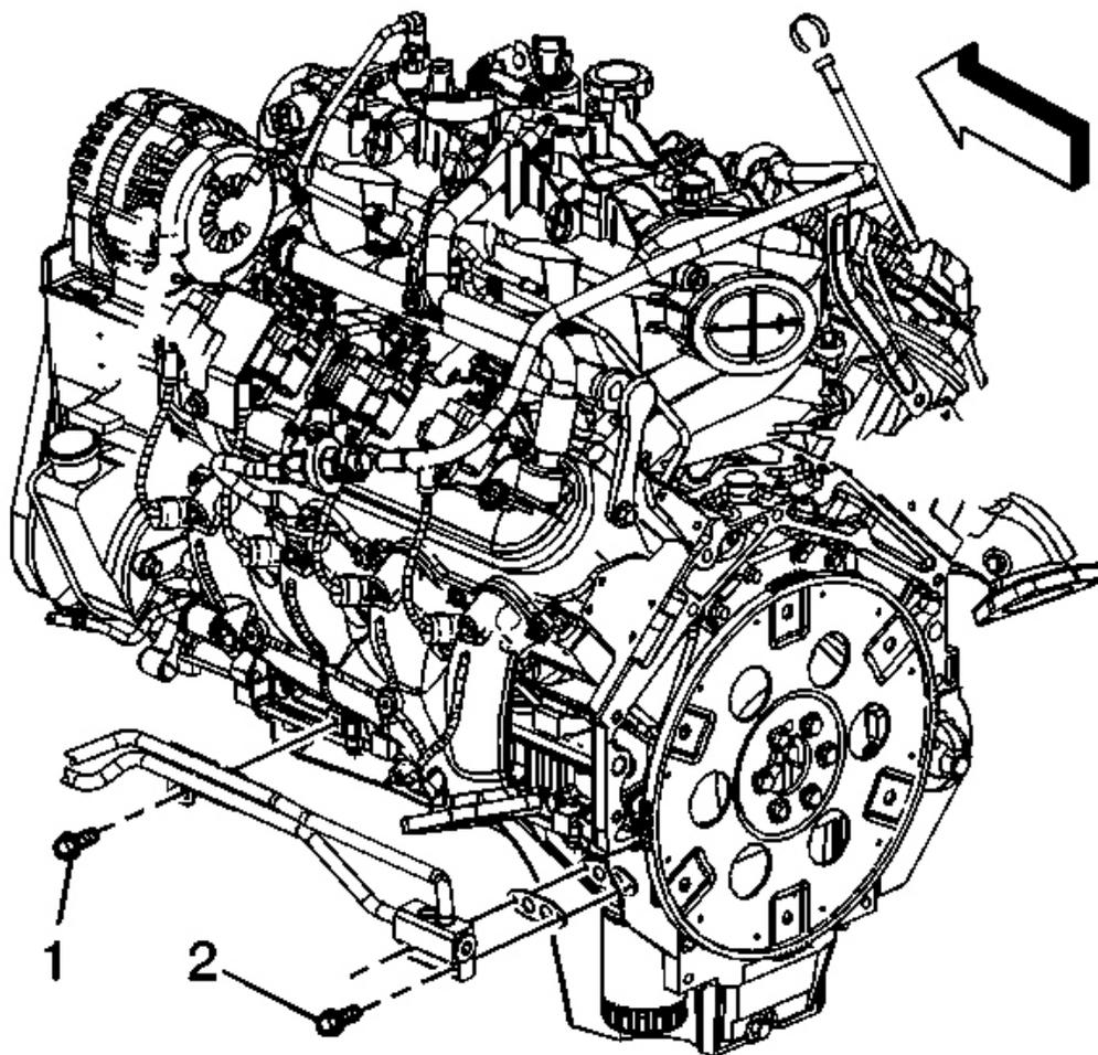
**Fig. 43: Oil Cooler Hose Bracket Bolt & Adapter Bolts**
