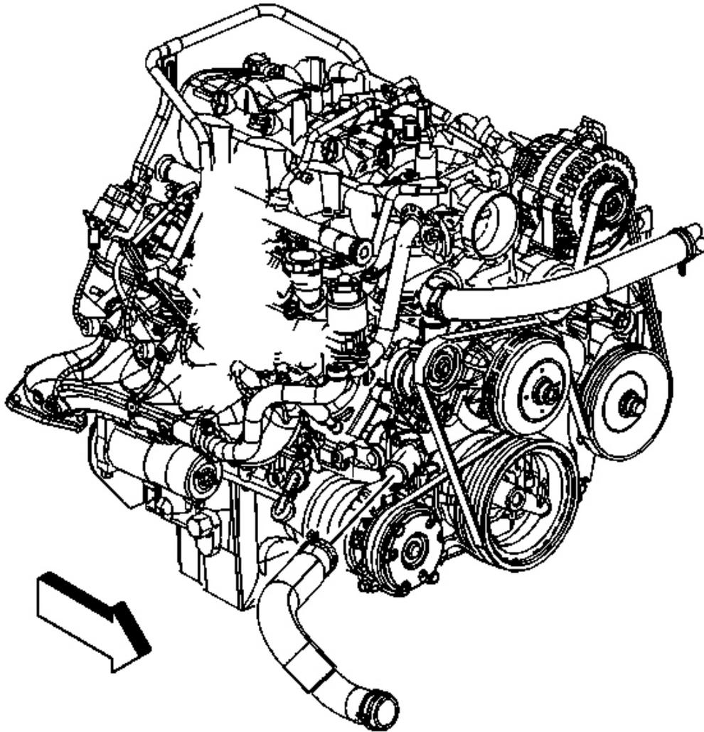
**Fig. 82: Outlet Hose & Water Pump (4.8, 5.3, & 6.0L)**
