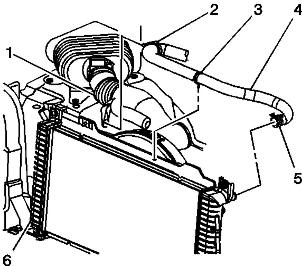
**Fig. 91: Radiator Hose & Radiator (Inlet)**
