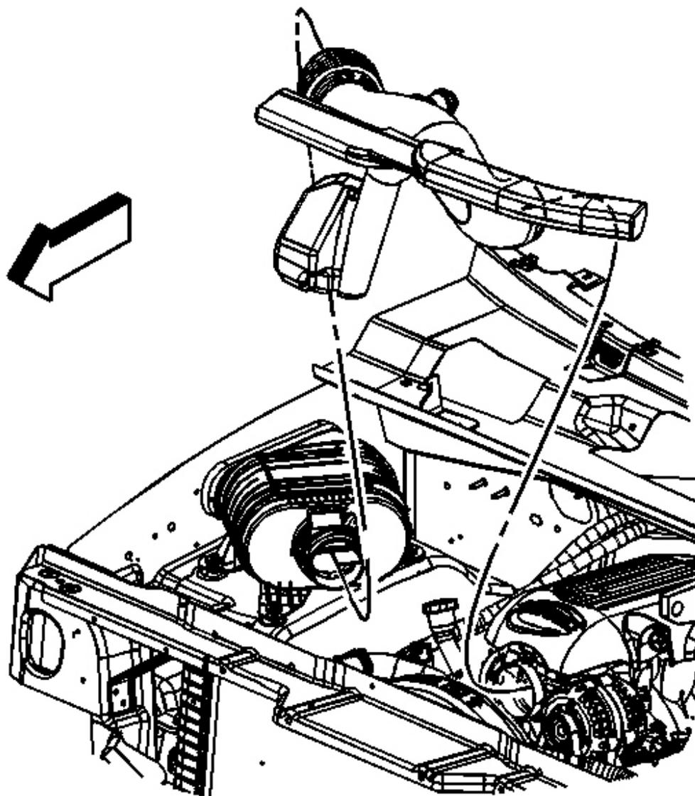
**Fig. 58: Air Cleaner Outlet Duct**
