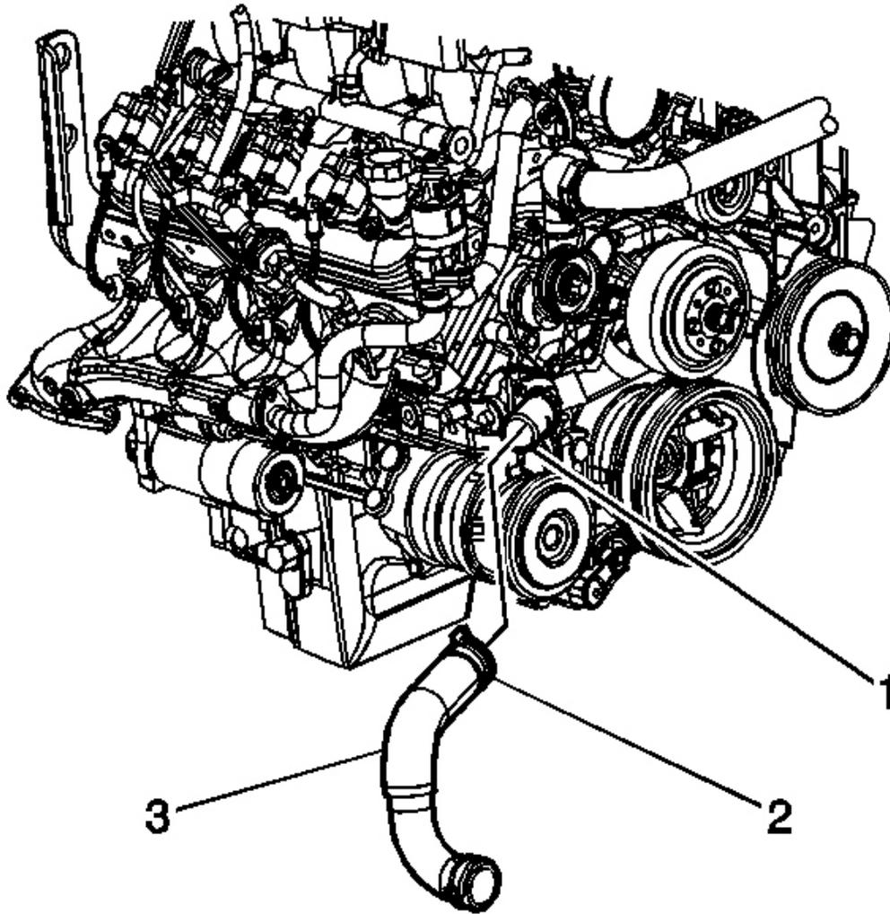
**Fig. 30: Radiator Hose & Engine (Outlet)**
