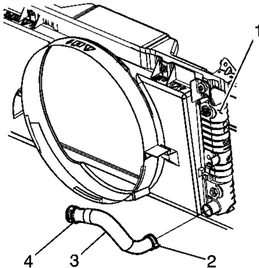
**Fig. 29: Radiator Hose & Radiator (Outlet)**
