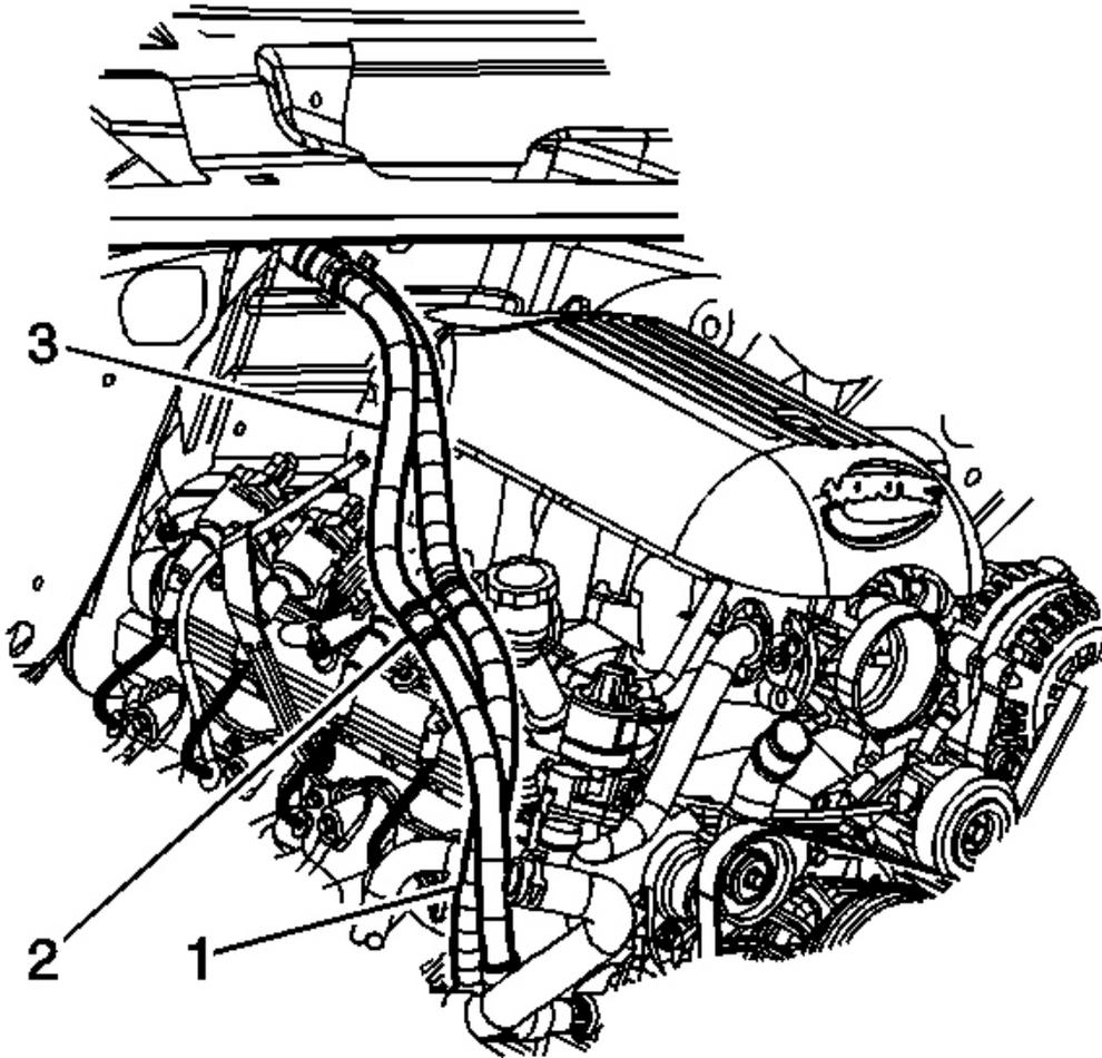
**Fig. 16: Heater Hose & Mounting Clip**
