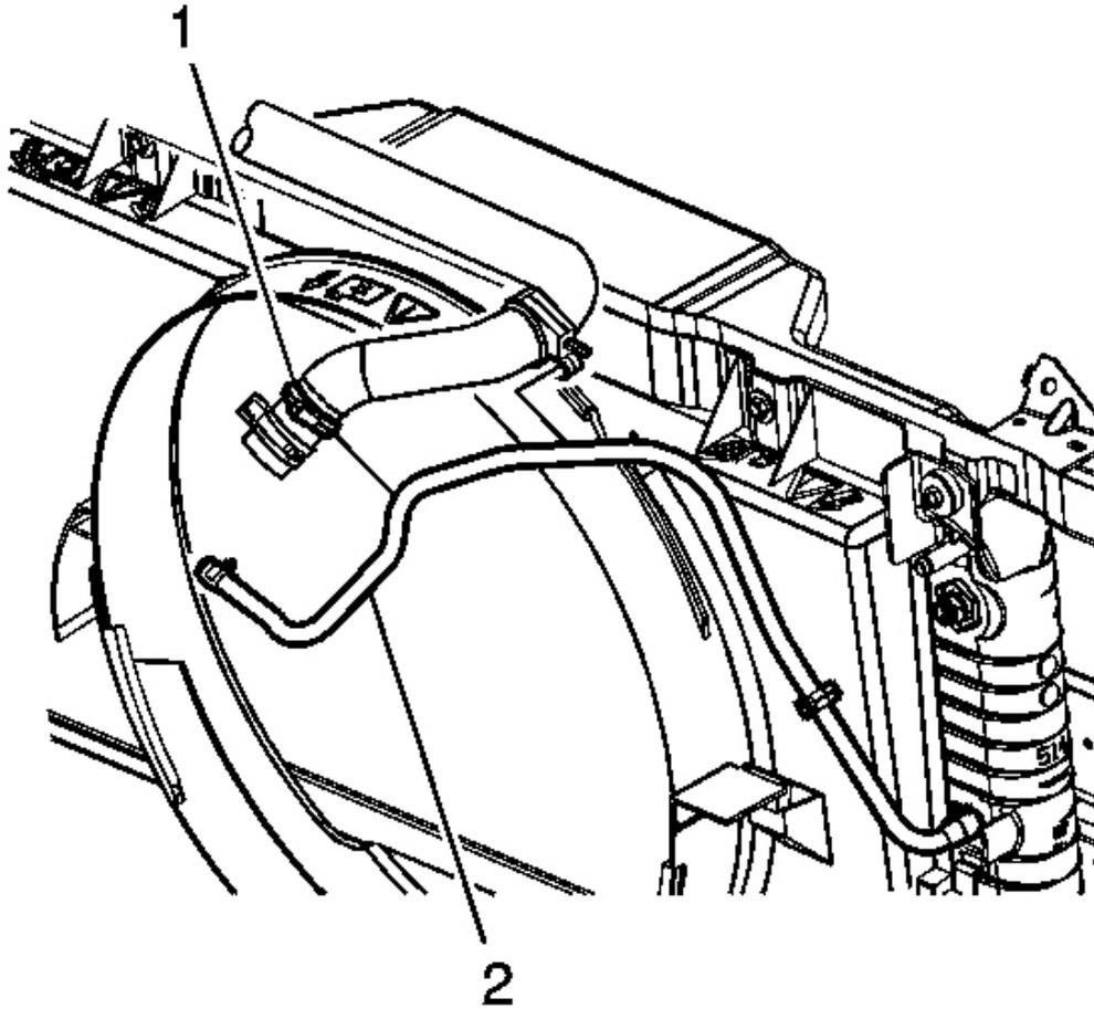
**Fig. 98: Radiator Vent Inlet Hose**
