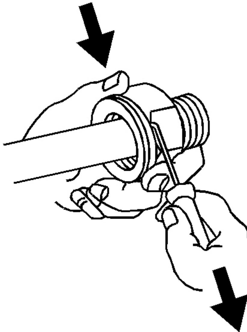
**Fig. 33: Rotating Retaining Ring**
