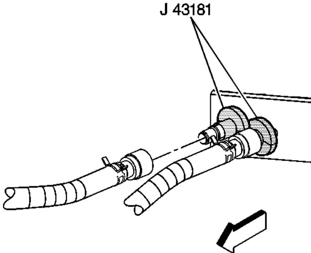
**Fig. 15: Identifying Heater Hose To Heater Core Outlet**
