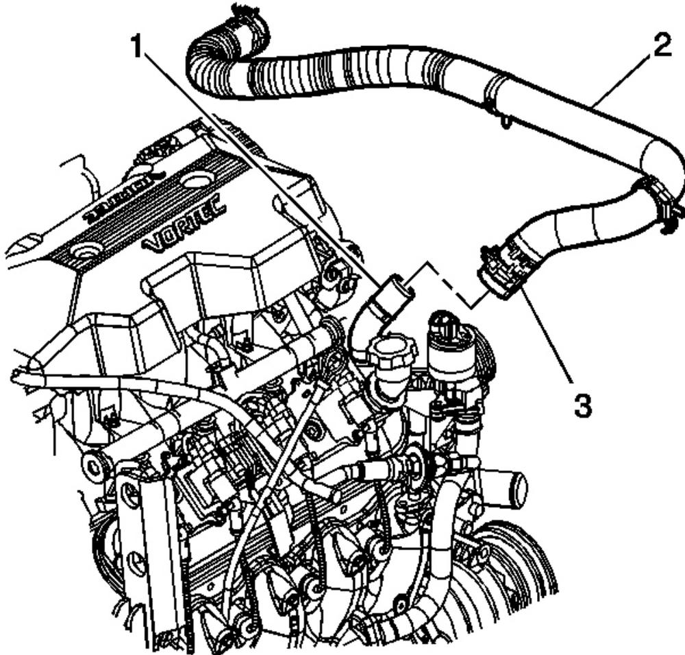
**Fig. 23: Radiator Hose & Engine (Inlet)**
