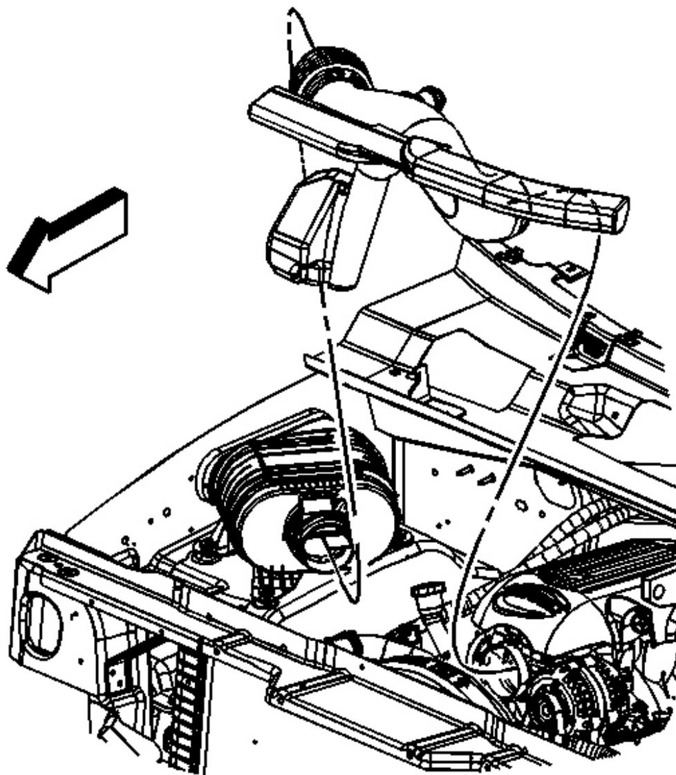
**Fig. 85: Air Cleaner Outlet Duct**
