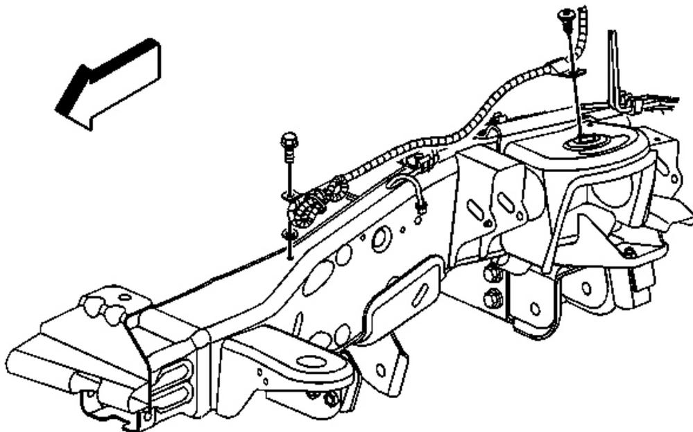
**Fig. 111: Engine Coolant Heater Cord**
