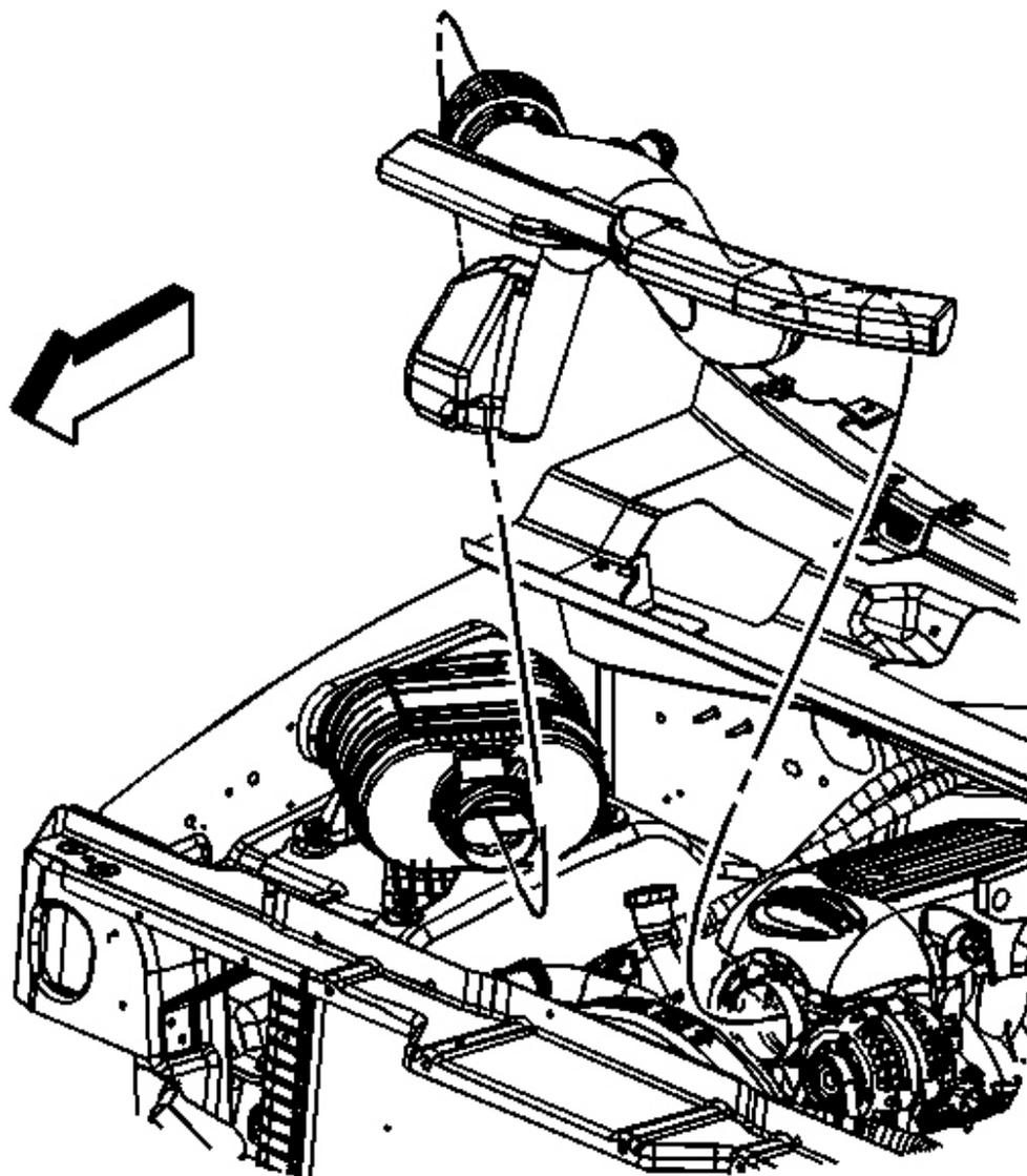
**Fig. 72: Air Cleaner Outlet Duct**
