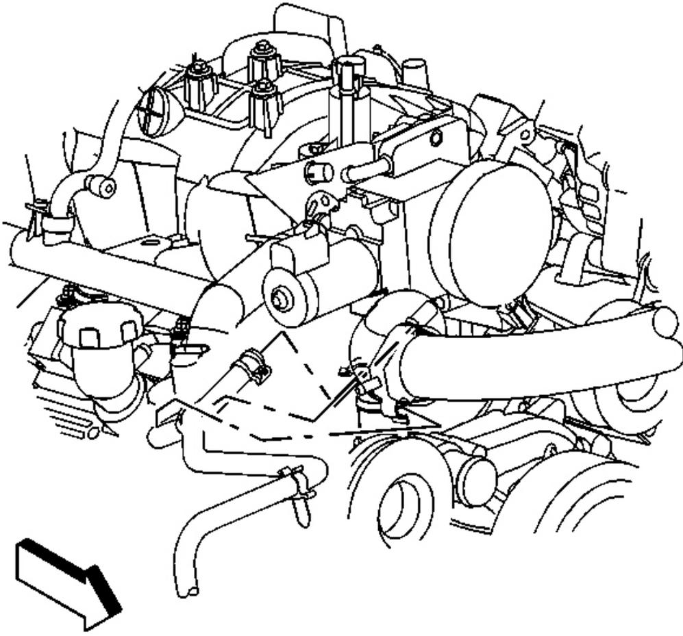
**Fig. 84: Vent Inlet Hose At Throttle Body**
