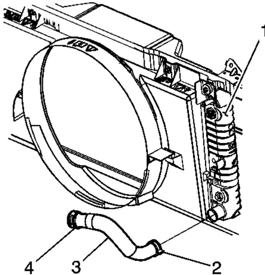
**Fig. 28: Radiator Hose & Radiator (Outlet)**
